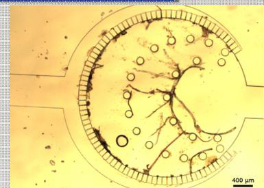
Fig. 7. A result of veterinarian measurement using the developed flow-thought nematode filter.
