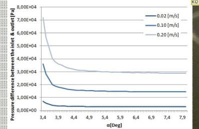
Fig. 6 Pressure difference between inlet and outlet as a function of angle  $\alpha$  at fix inlet velocities (0.02 m/s, 0.1 m/s, 0.2 m/s).
