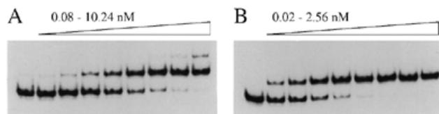
**Figure 3.** Protein titrations showing that the target site recognition is strongly context dependent. The RR<sub>TRPS</sub> mutant binds  $O_{R1-2'A1'A}$  operator (B) ~15-fold better than  $O_{R*1}$  (A).
